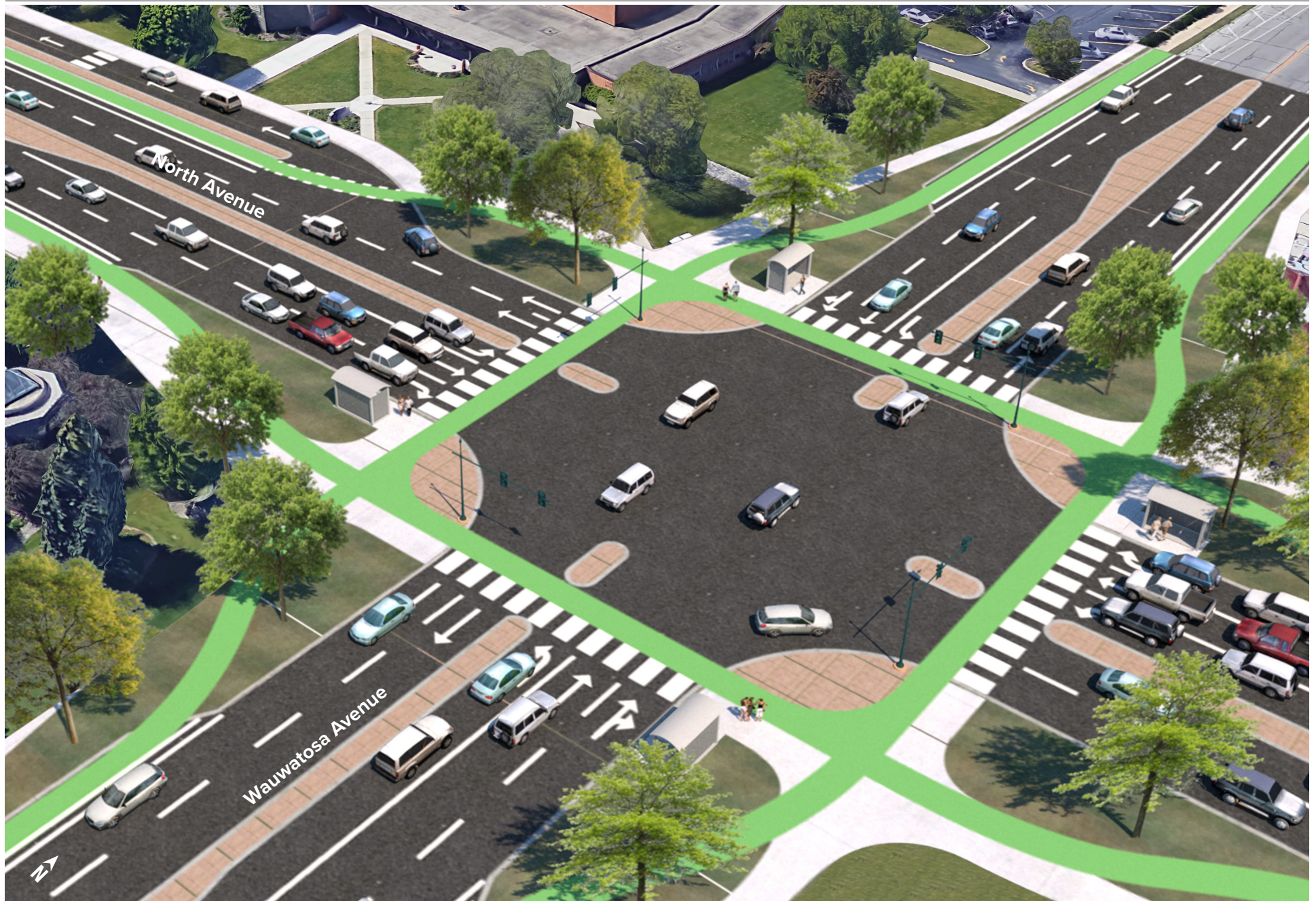
Figure 4.11: Wauwatosa Avenue Protected Intersection
